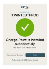
The Charger will attempt a network connection, if successful will then reboot to complete an RCD and safety function check.
