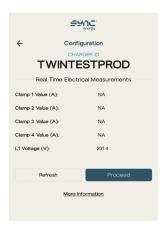
Check the shown electrical measurements match the measured readings. This will allow checking the load management CT is fitted in the correct orientation and location. A negative value indicates reverse direction of power due to, e.g Solar surplus, but could also indicate that the clamp has been installed in a reversed (incorrect) orientation or polarity wiring.
