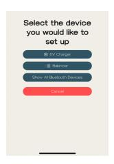
2 Ensure Bluetooth is activated on your device, and select set up new product. If the EV charger does not show up under EV Charger option, go back and select show all Bluetooth devices. If no Bluetooth devices are shown, please check Bluetooth is turned on and the permission was granted in the app.
