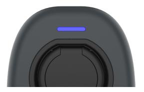
In less than 2 minutes, the indicator should turn from Yellow to Blue to confirm network connection.
