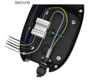
For dynamic load balancing, insert wires into the small connector
