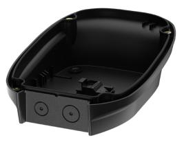
Rear cable entry - Suitable for 25mm hole size Base cable entry - suitable for 16-32mm hole size
