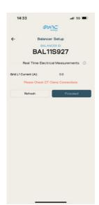
**Please Note:** A minimum of 3 amps is required to ensure correct CT connection, Press Refresh to retrieve the latest readings.
