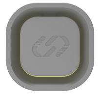
Upon powering the charger, the status indicator light will show **Yellow**. This indicates that the charger is ready for network setup but is not yet connected to the internet. These steps are still required for 4G connected versions for setting of Dynamic Load Management.
