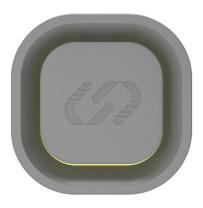
Upon powering the charger, the status indicator light will show **Yellow**. This indicates that the charger is ready for network setup but is not yet connected to the internet. These steps are still required for 4G connected versions for setting of Dynamic Load Management.
