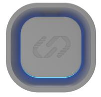
In less than 2 minutes, the indicator should turn from Yellow to Blue to confirm network connection.
