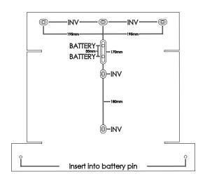
Screw inverter bracket to wall ensuring bracket sits flush and bracket is secured
