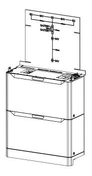
Screw inverter bracket to wall ensuring bracket sits flush and bracket is secured
