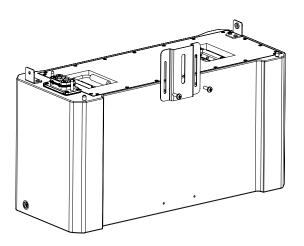
Stack batteries (maximum of 4 for this configuration) however do not stack the last battery, on the 2nd to last battery add the drill template, this needs to be inserted into the 2 pegs, drill holes marked BATTERY and insert wall plugs if needed
