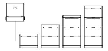
Option B - One tower - consisting of inverter and up to 15kwh of batteries
